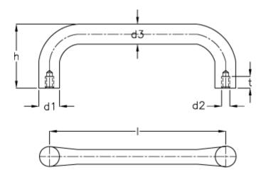
$$\begin{array}{ll} d1 & = 25 \\ d2 & = M12 \\ d3 & = 18 \\ h & = 59 \\ I & = 140 \\ t \ min = 20 \end{array}$$
